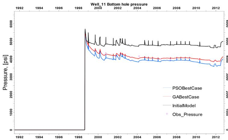
Figure 2: History matching of bottom hole pressure of well 11.
