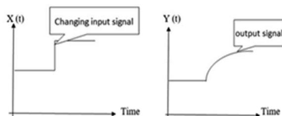
Figure 1: Effect of time constant on output signals.
