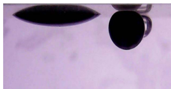
Fig. 4 The change in the contact angle from the initial state [left] to the equilibrium [right] for high adsorption foam.
