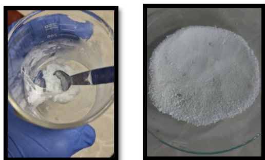
Fig. 2 Water extraction and polymer drying steps (from right to left).
