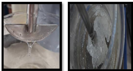
Fig. 1 Synthesized polymer solution with a concentration of 10% (left: oxidation-reduction method, right: thermal method).
