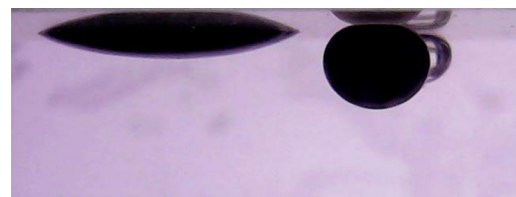
Fig. 4 The change in the contact angle from the initial state [left] to the equilibrium [right] for high adsorption foam.
