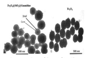
Figure 1: TEM image of the Fe<sub>3</sub>O<sub>4</sub>/Guanidine
