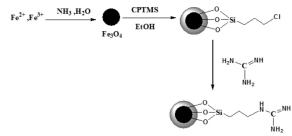
Scheme 1: the reaction between Fe<sub>3</sub>O<sub>4</sub> and guanidine
