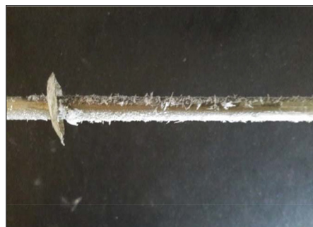
Figure 1. Needle solid crystalline which was formed around the reactor thermo-well.
