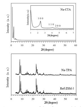
Fig. 1: XRD patterns of the reference and desilicated HZSM-5 samples. References
