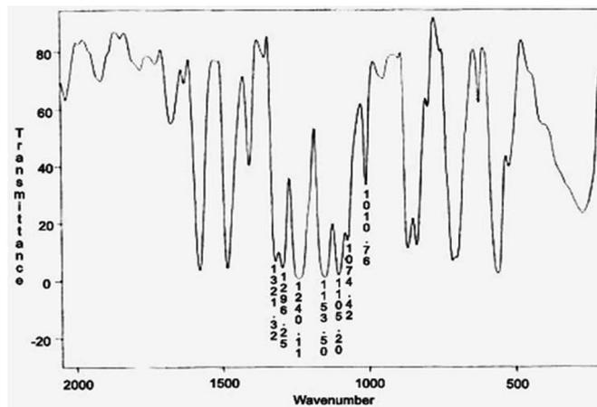
Figure 1: FTIR spectra of composite membranes filled with  $\text{SiO}_2\text{-SO}_3\text{H}$  nanoparticles
