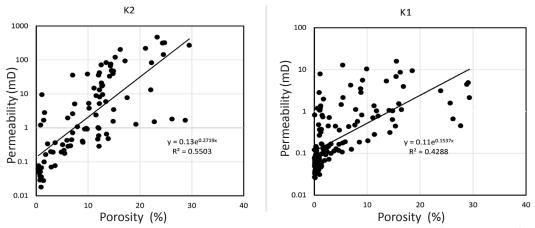
Figure 1: Permeability-porosity relationship in the reservoir units K1 and K2 of the Kangan formation.
