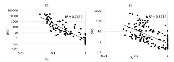
Figure 2: The *DRQI* values, computed using equation (4), versus  $S_w$  data in the reservoir units *K1* and *K2* of the Kangan formation.
