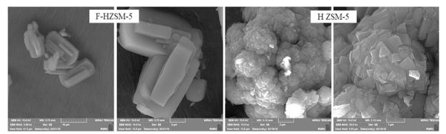
Figure 1: FESEM images of HZSM-5 and F-HZSM-5 zeolites.
