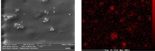
Figure 2: a) SEM image and b) EDX analysis of PES/TiO<sub>2</sub> membrane surface.
