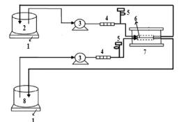
**Figure1:** Schematic diagram of forward osmosis system: 1)Digital mass balance, 2)Feed solution, 3)Pump, 4)Flow meter, 5)pressure gauge, 6)membrane, 7)FO membrane cell, 8)Draw solution.
