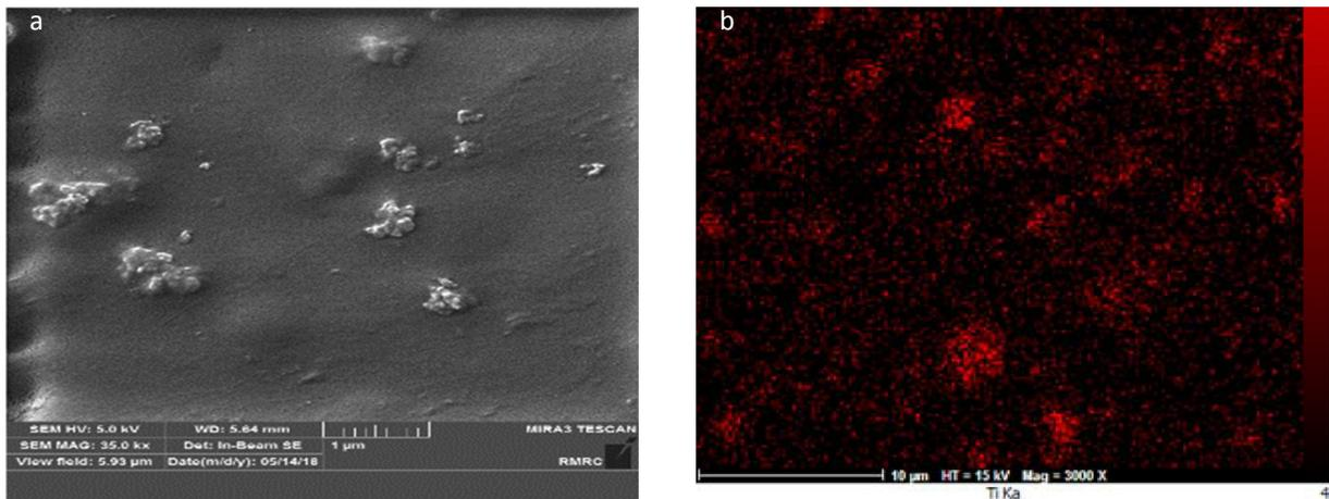
Figure 2: a) SEM image and b) EDX analysis of PES/TiO<sub>2</sub> membrane surface.
