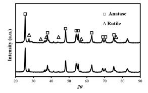
Figure 1: XRD patterns of TiO, and N-doped TiO,.
