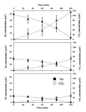
**Figure 4:** The photocatalytic conversion of n-Hexane over N-doped  $TiO_2$  sample under visible-light illumination by varied n-Hexane (Hx) concentrations.
