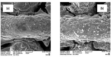
Figure 2: SEM images of the coated stainless steel webnet supports with, (a) TiO<sub>2</sub> and (b) N-doped TiO<sub>2</sub>.
