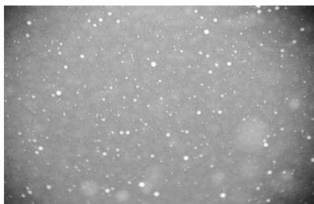
**Figure 3 b:** Microscopic Image of Heavy Hydrocarbon in Water Emulsion.
