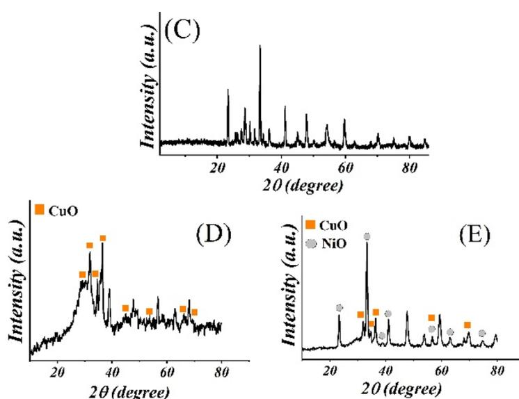
**Figure 1:** The XRD patterns of (C) ZnLaAlO<sub>4</sub> support, (D) Cu/ZnLaAlO<sub>4</sub>, (E) Cu-Ni/ZnLaAlO<sub>4</sub> catalysts.
