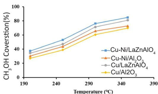
**Figure 2:** Comparison of methanol conversion using synthetic catalysts.
