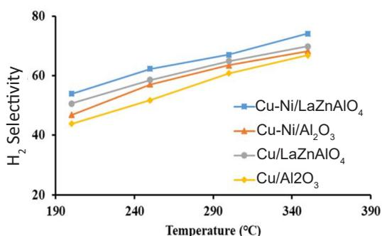
observed that by increasing the temperature, the possibility and amount of CO formed increased. This is in conformity with CO production mechanism via reverse water-gas shift reaction since rising temperature increases methanol conversion and thus increases concentrations of hydrogen and carbon dioxide, the reactants in water-gas shift reaction, in the reactor and the possibility of CO formation.
