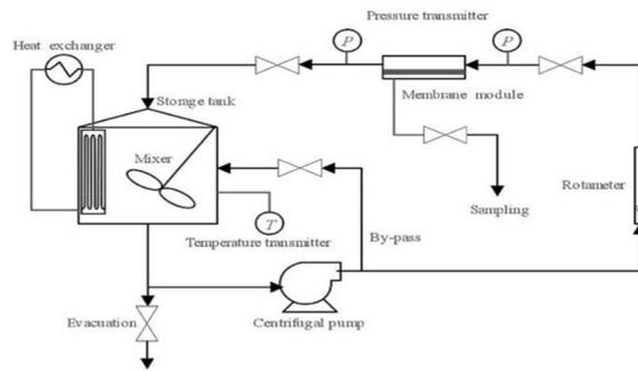
Figure 2: Microfiltration setup
