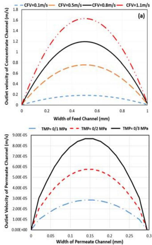
**Figure 5:** Effects of CFV and TMP on velocity profile at outlet (a) concentrate channel (b) permeate channel.
