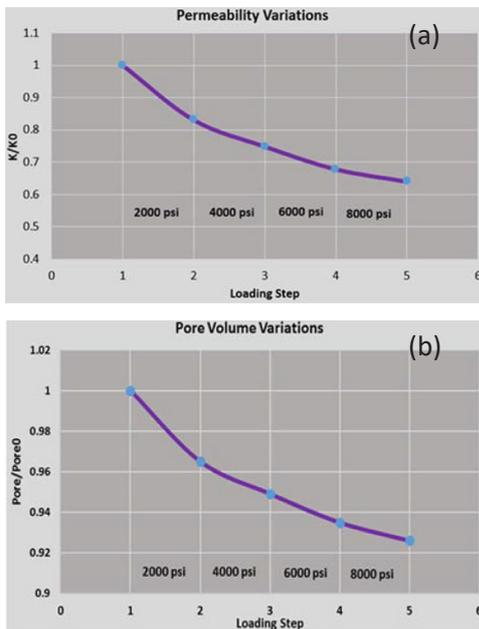
**Figure 2:** The trend of normalized permeability (a) and pore volume variations (b) under loading of sample.
