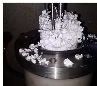
Figure 2: Methane hydrate picture formed under the cooling rate of 10 °C/h (top (or above) image) and 5 °C/h (down (or below) image) at the blank tests.
