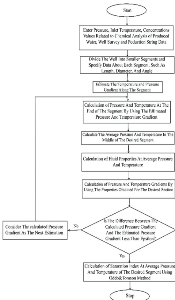
Fig. 1 Calculation algorithm for calculation saturation index in the well.
