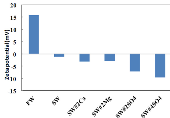
Figure 1: The results of the Zeta potential versus the type of smart water and formation water.
